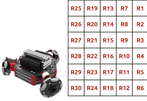
Fig. 1. Rosie HEBI mobile base (left) and workspace discretization (right).
