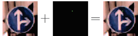
Figure 1: An adversarial example for a neural network trained on the GTSRB dataset. After a slight perturbation, the image classification changes from “go right or straight” to “go left or straight”.
